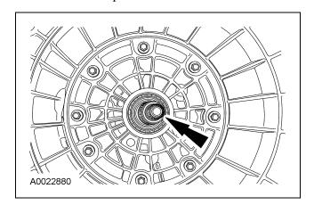
112. Using the special tool, make sure that the fluid pump gear seal ring is fully seated.
